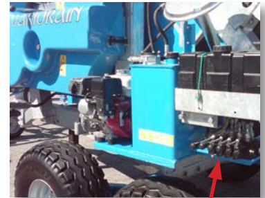
Optional hydraulic Honda engine drive with 4 levers (reel, stabilizer legs, tongue jack and turntable)
