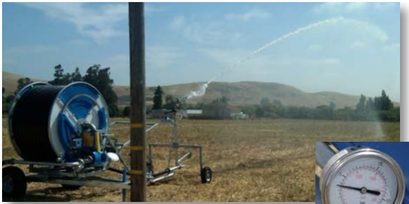
OCMIS machines require less pressure - this machine is running at 52 psi at the inlet
