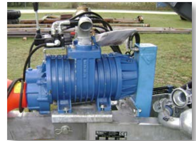
Optional blow-out compressor -- cleanse out water in hose in 3 min.
