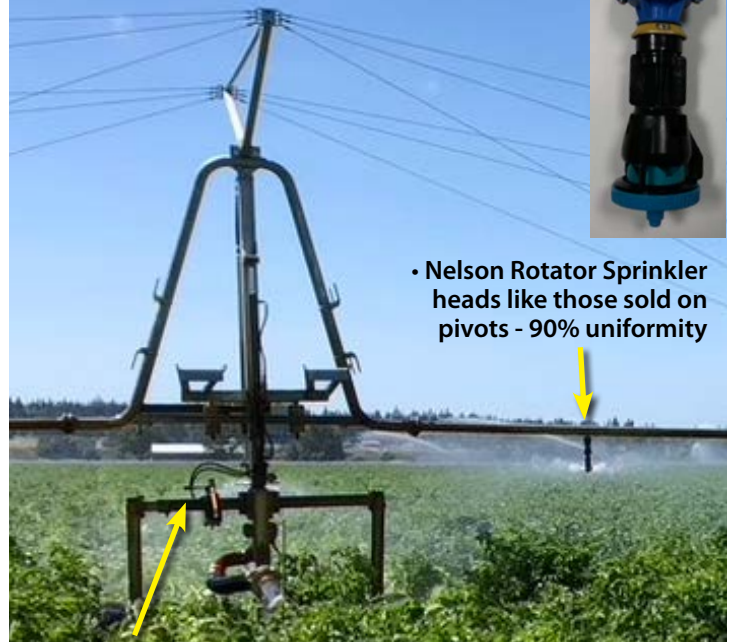
• Optional hydraulic lift to raise and lower the boom - up to 8' tall!
