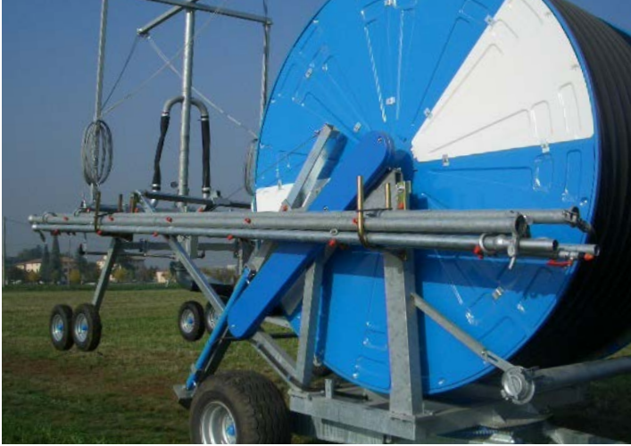
• Easy to transport - pipes stack on the side of the reel
